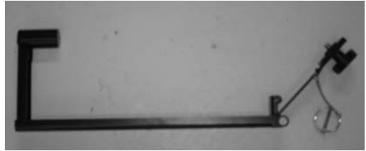
(2) Remove locking pin on the pivoting arm
