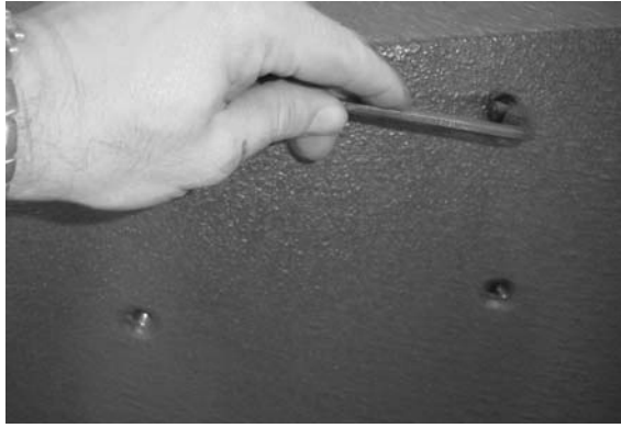
(1) Remove Omnimount attachment screws (5 mm allen key)
