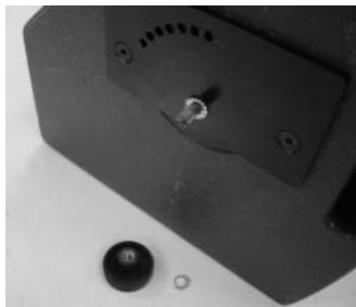
(7) Remove ETRI attachment knob and lock washer
